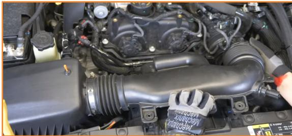
10. Remove the bolts that secure the vacuum pump to the bracket. Do not remove the pump.
