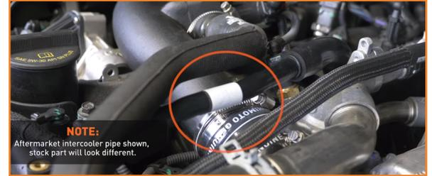
5. Squeeze the quick-disconnect fittings at each end of the crankcase breather hose, and then remove the hose.
