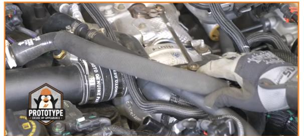
15. Connect the Mishimoto outlet hose to the PCV heater and push the yellow tab to secure the connection. The fitting should click twice.
