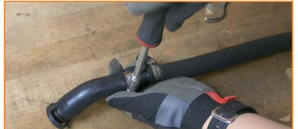
14. Route the hose with the rubber elbow under the bypass valve pipe and connect it to the valve cover. Route the other end under the turbocharger muffler and connect it to the IN port on the catch can. (1x worm gear clamp)
