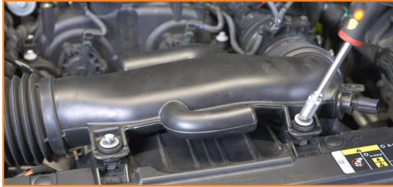
8. Loosen the clamps on that hold the intake pipe on the turbocharger muffler and the airbox. (2x worm gear clamps)
