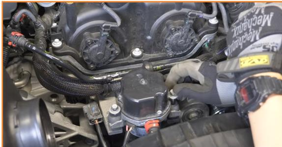
11. Lift the vacuum pump slightly so that you have enough room to slide the catch can bracket under the pump. Align the holes in the bracket with the pump's grommets. With the bracket set, secure the bump using the original hardware. (2x 10mm bolts)
