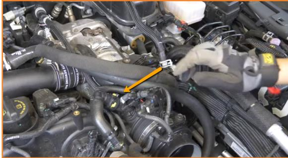
16. Connect the other end of the outlet hose to the OUT port on the catch can. (1x worm gear clamp)
