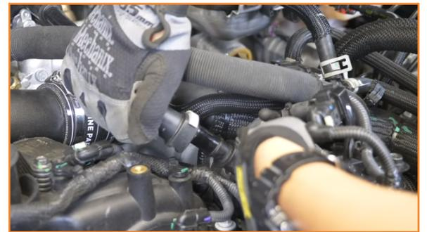
6. Separate the intake air temp sensor wiring from the intake pipe. Next, disconnect the sensor electrical harness from the intake.
