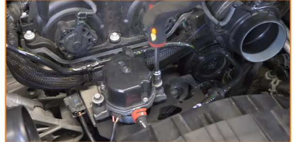
12. Secure the catch can to the bracket with the fittings facing away from the pump. (3x 2.5mm Allen bolts)
