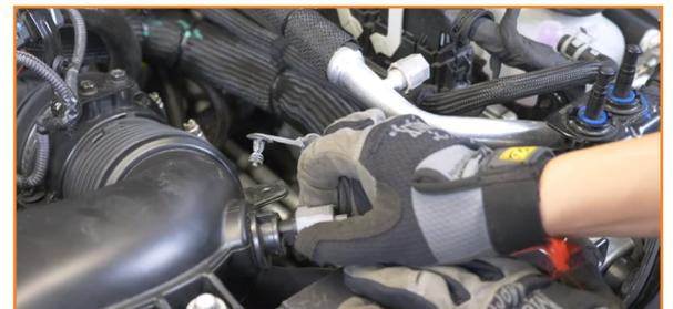
7. Remove the bolts that secure the intake brackets. (2x 10mm bolts)
