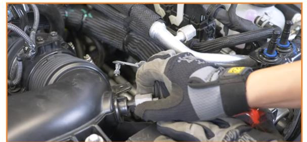
7. Remove the bolts that secure the intake brackets. (2x 10mm bolts)
