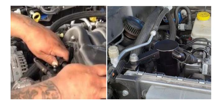
Always check and drain the catch can more often in winter / freezing weather. If the water/oil mixture in the catch can is allowed to freeze it will cause damage to the catch can and internal components. Any damage due to freezing is NOT WARRANTY.
