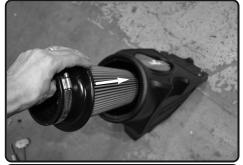
11. Install the twist lock filter into the airbox and secure.
