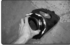
**12.** Once the twist lock filter is seated properly, rotate the filter in either direction a 1/4" turn untill filter locks into place.
