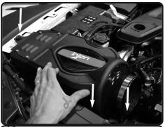
**13.** Install the airbox assembly into the vehicle. install into the factory position. Secure using the OEM screw from step
