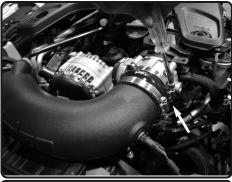
**16.** Secure and tighten all the clamps on the intake tube using 8mm nut driver.
