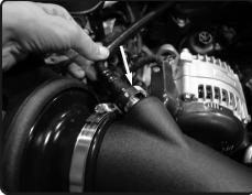
**15.** Connect the crank case vent tube to the machined fitting on the intake tube.
