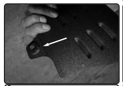
**9.** From step 4, install the grommet with crush washer to the hole on the airbox bracket.
