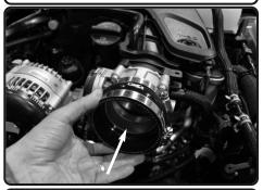
**8.** Install the provided step hump hose to the throttle body. Secure using provided clamps.
