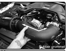
**14.** Install the provided rubber grommmet to the intake tube hole. Insert the Injen intake tube into the vehicle. Position tube to the filter and throttle body. Postion for best fit.
