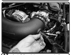
**17.** Install the air temp sensor to the rubber grommet on intake tube and reconnect the harness.
