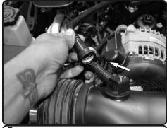
**6.** Disconnect the crank case line from the intake tube.
