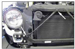
7. Remove the two bolts that secure the core support brace to the core support and remove
