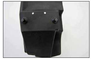
11. Install two airbox mounts onto the K&N® airbox with provided hardware.
