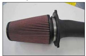
14. Install the K&N® air filter onto the K&N® intake tube.
