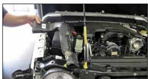
8. Remove the two bolts that secure the inlet scoop to the core support and remove inlet scoop.
