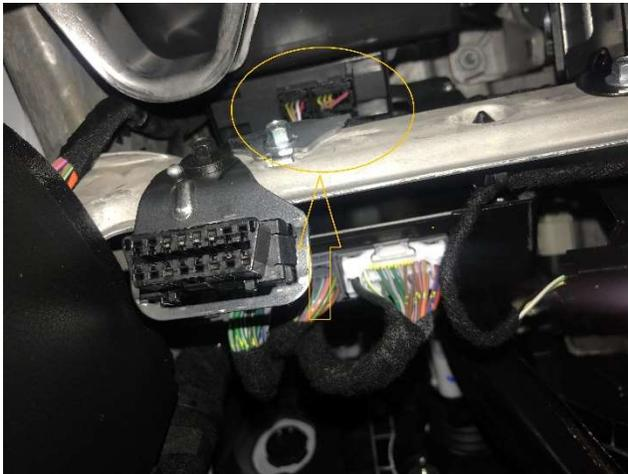
Once the SGW bypass is plugged in, you can plug the Tazer JL into the OBD2 diagnostic port under the dashboard, on the left side. The Tazer JL does not need to be plugged in for any of the features in the *Vehicle Settings* to remain operational. The Tazer JL can be left plugged in, as many of its
