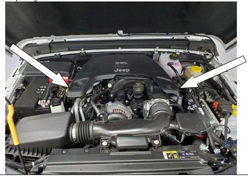
Locate the PCV line that runs from the rear of the passenger side valve cover to the driver side of the intake manifold. Push grey tab and pull from fitting. Remove entire hose from engine and save.
