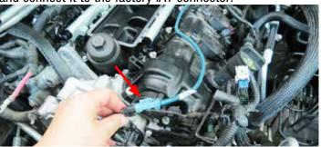
68. Apply o-ring lube to the o-ring on the supplied MAP sensor and carefully install it into the front provision on the intercooler adapter. Apply blue thread locker onto the threads of the M4 x 16mm bolts and secure the MAP sensor to the intercooler adapter using a 3mm Hex Key. Torque the bolts to **18 in. lbs**. DO NOT OVERTIGHTEN.
