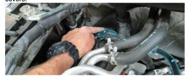
25. Remove the quick-connect ends off of the factory driver side PCV hose by carefully cutting the plastic hose with a razor.
