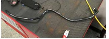
26. Insert the quick-connect fittings into the supplied 43" hose. TIP: Heating the hose will help in the insertion of the fittings.
