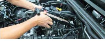
21. Using a shop vac or clean shop rag, clean the cylinder head flanges and cover the ports with protective tape.
