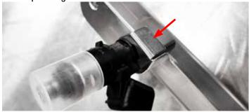
63. Install the 45° fitting on the supplied fuel crossover onto the rear driver side fuel rail fitting. Install the other end of the crossover onto the passenger side rail fitting AFTER the fuel rails have been installed on the manifold. (Step 67) This is done so the fuel line can be routed around factory wire harnesses and coolant lines.
