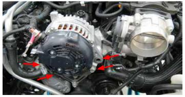
11. Undo the two bolts on the intake manifold to support bracket using a 10mm socket.
