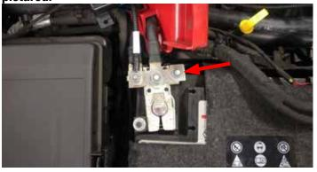
89. Using a 10mm socket, connect the Ground (-) wire on the water pump harness to the chassis ground located between the battery and fender on the passenger side fender. **NOTE:** Use the fastener without a factory cable attached as pictured.
