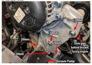
54. Using two M8 x 30mm hex flange bolts from Bag #1, install the alternator onto the FEAD bracket. Using one of the longer factory alternator bolts, secure the alternator to the lower-left factory provision. Torque M8 bolts to 22 ft-lbs (30 Nm) and the stock bolt to 41 ft-lbs (55 Nm).
