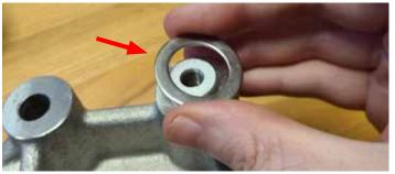
56. Position the alternator support bracket spacer, support bracket, and a M8 x 40mm hex flange bolt from Bag #1 onto the supplied 70mm pulley as shown. Apply blue thread locker to the threads of the bolt and loosely install it onto the upper FEAD provision as shown.
