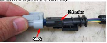
74. Connect the MAP extension harness to the MAP sensor located on the front of the upper manifold.
