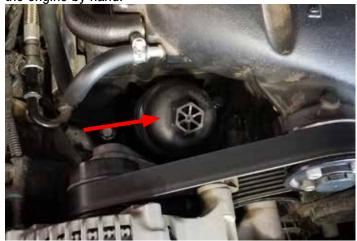
Once the oil has been drained and the drain plug reinstalled, place a long funnel into the cannister filter orifice as pictured here. Add oil as recommended by the manufacturer.
