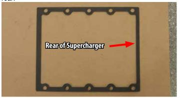
80. Carefully lower the supercharger onto the upper manifold and verify that the gasket is properly aligned. Apply blue thread locker onto the threads of the ten (10) M8 x 22 SHCS bolts from Bag #3. Install the bolts and fasten using a circular sequence starting with the inner bolts and working outwards. Torque the bolts to 18 ft-lbs (24.4 Nm). Once secure, install the factory hard line to the EGR valve. Reconnect the EGR valve electrical connector.
