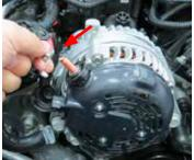
10. Using a 15mm socket, remove two (2) upper bolts securing the alternator to the engine. Remove two (2) lower bolts securing the alternator to the bracket using a 13mm socket. **NOTE:** One of the 15mm bolts will be reused.
