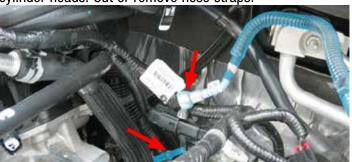
23. Install the 90° end of the supplied fuel feed line to the factory hard line. Route fuel line through the hoses behind the engine to be able to reach the front of passenger side intake flange.
