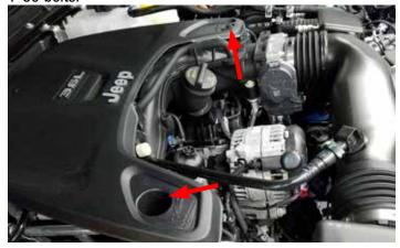
Remove two bolts from front of vehicle on the intake tube using a 10mm socket (will be reused). Be sure to also remove the PCV hose, disconnect the IAT sensor, and remove the 3 harness clips on the intake tube before removing. **NOTE:** The IAT sensor pictured here will not be reused. Leave the sensor installed to seal the port.
