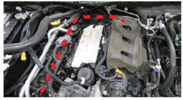
29. Install the supplied passenger side PCV hose to the rear of the passenger valve cover. Route the hose under the coolant lines. Hose will connect to the supercharger later.
