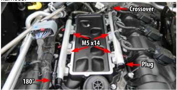
66. Connect the injector electrical connectors to the proper injectors. Position the fuel feed line around the passenger side fuel rail and connect it to the 180° fuel fitting.
