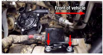
43. Place the surge tank bracket over the coolant lines' front mounting point using the factory bolt. Using two M6 x 10mm bolts from Bag #2, secure the surge tank to the surge tank bracket.
