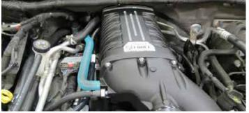
Connect the supplied EVAP hose to the EVAP solenoid. Connect it to the smaller fitting located towards the front of the supercharger on the passenger side. Trim hose to fit.
