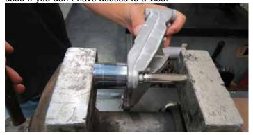
46. Carefully install the bushings into the supplied FEAD bracket using a vise or equivalent. WARNING: DO NOT use a hammer as it may damage the bushings and/or FEAD bracket.
