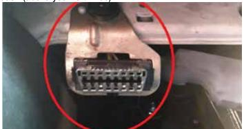
3. Directly behind and above the OBDII connector, locate the security bypass module. Disconnect the larger of the two connectors.
