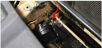
40. Secure LTR brackets to the LTR using (4) M6 x 10mm bolts from hardware bag #2. Then, install the assembly onto the core support using the factory hardware where the original braces were located. Connect horn extension cables to the factory horn leads and route behind the LTR. Reconnect the horns and replace the upper bumper cowl.
