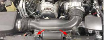
5. Remove the 10mm bolt holding the airbox to the fender. Remove the box and intake tube assembly and set aside.
