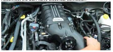
81. Using a 1/2" breaker bar, rotate the hydraulic tensioner clockwise and finalize the installation of the drive belt.
