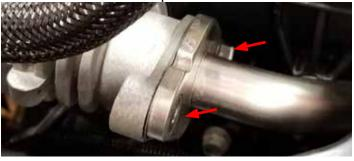
14. Twist lower oil fill neck by depressing the locking tab and lift up. Remove cap and reinstall cap onto lower oil fill. **NOTE:** Once the supercharger is installed, there will be no access to this oil fill cap. The oil filter cartridge port will be used as the oil fill.
