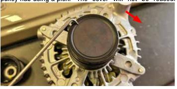
48. Using a 17mm Allen socket and impact wrench, remove the alternator pulley CLOCKWISE. This pulley has a left-handed thread. Use the impact wrench in short bursts to remove. This pulley will not be reused.
