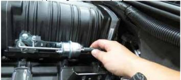
85. Remove the factory throttle body 0-ring from the manifold and clean using a shop rag. Install the gasket onto the supercharger throttle body flange as shown.
