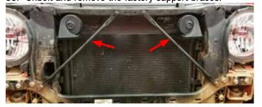
34. Remove the (2) T20 screws holding the lower air scoop onto the core support.
