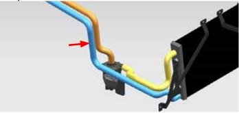
42. Connect the water pump harness to the pump. Install the water pump and water pump bracket onto the power steering motor using supplied M6 x 10mm bolts in bag #2 on the passenger side. Clock the water pump so the outlet is pointing towards the front of the vehicle.
