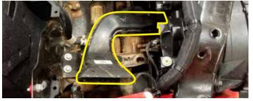
36. Unbolt the factory horn brackets located on the upper core support facing the radiator. Unplug and set aside. **NOTE:** Jeeps optioned with oil cooler will need to loosen the 2 top bolts of the radiator to access the horn bracket bolts.
