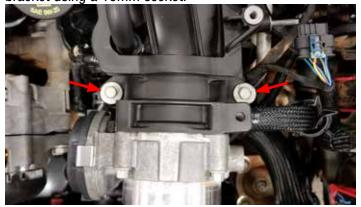
12. Disconnect EVAP, Brake Booster, Driver' Side PCV hose, and MAP sensor from intake manifold and slide EVAP solenoid and isolator off intake manifold.
