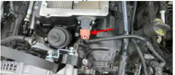
75. Connect the supplied bypass actuator hose to the barb located on the rear of the upper manifold. This will connect to the bypass actuator once the supercharger housing is installed.
