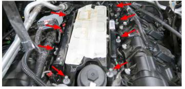
20. Carefully remove the lower manifold and set aside.
