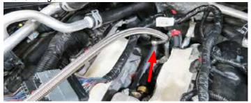
24. Remove both PCV hoses from the rear of both valve covers
