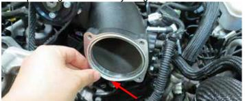
86. Secure the throttle body to the supercharger nose using four (4) M6 x 40mm hex flange bolts from Bag #3. Reconnect the throttle body electronic connector.
