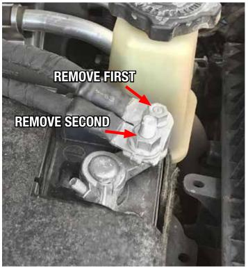
Reconnect after 30 minutes. First, connecting the cable attached to the terminal clamp. Secondly, connecting the cable that attaches to the stud.
