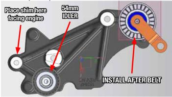
52. Feed the drive belt down towards the crank. Using the belt routing diagram, route the belt around the P/S, tensioner, crank, water pump and A/C.
