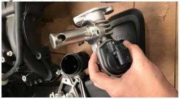
77. Remove the EGR O-ring from the original intake manifold and insert into the supercharger nose EGR provision.
