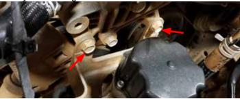
Using ½" breaker bar and extension, remove tension from the belt (clockwise) and slide the belt off the smooth idler. Belt will not be completely removed at this time.
