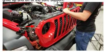
33. Unbolt and remove the factory support braces.
