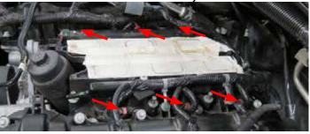
19. Using an 8mm socket, remove eight (8) bolts securing the lower manifold to the cylinder heads. Uninstall (3) harness clips located in the rear of the manifold.
