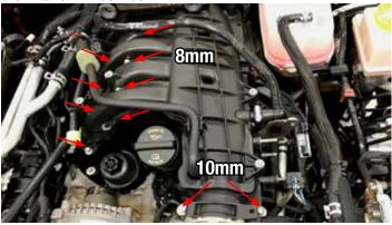
16. Clean any debris from around the port openings and cover the port openings with tape. Remove the foam insulator. It will not be reused.
