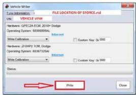
20. Once the flash is completed, click CLOSE, turn the ignition OFF and disconnect the RTD from your OBDII port. The engine is now ready to start once the supercharger installation is complete!
