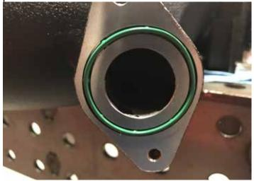
78. Install the EGR to the Supercharger nose using the supplied M6x20mm bolts. Use the factory bolts on the hardline mounted on the rear of the EGR.
