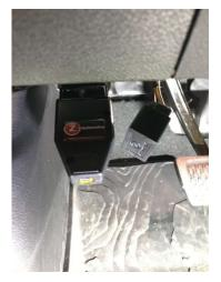
features (*Live Functions*) only work when plugged in. The Tazer JL will go to sleep by itself, 30 seconds after the car shuts down.
