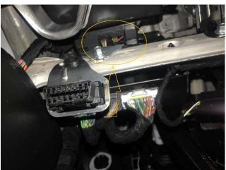
the wires. Once the SGW bypass is plugged in, you can plug the Tazer JL into the OBD2 diagnostic port under the dashboard, on the left side. The Tazer JL does not need to be plugged
