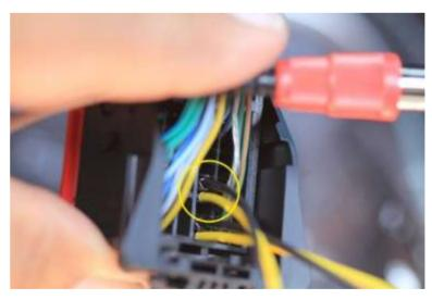
Once the cover is raised, plug the yellow wire's pin of the supplied RCA cable into slot 24, and the black wire into slot 25. They should snap into place. Once installed, re-seat the red terminal locking plate.
