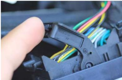
Unlatch the large radio connector arm and raise the arm to release the connector.
