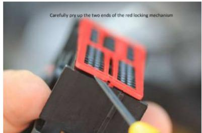
Using a small flat head screwdriver, raise red terminal locking plate off the main radio connector.
