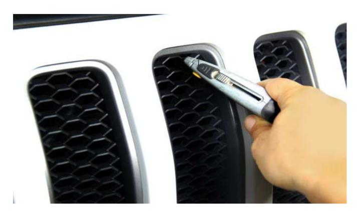
Using a box cutter or wire snips, trim middle grill slating to fit camera bracket
