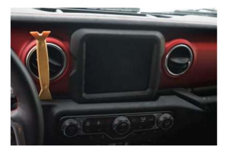
Step 2: Radio Bezel Removal
