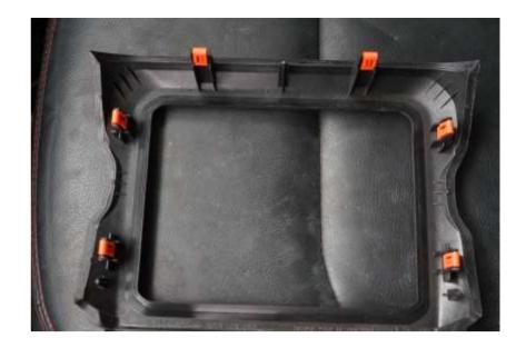
Once screws are removed, use a trim stick to remove bezel from dash.
