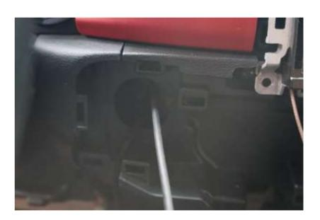
Using the wire routing diagram, run the camera wiring down the front of the vehicle and against the fender. The rear washer nozzle tubing hold down can be used to hold the camera wiring also. Run the wiring through the clutch plug and into the vehicle. Route under the dash and through the Push to start wiring hole. NOTE: It may be easier to first run the wiring through the firewall from inside the vehicle. Make sure to run wiring through clutch plug before running to the grill.
