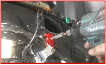
Install the ReadyLIFT rear bump stops to the axle using the provided  $1/4'' \times .75''$ bolts, washers, and nuts. Torque to 5 ftlbs (69-6835 kit number bump stops do not have R logo and are only 2.5" tall)
