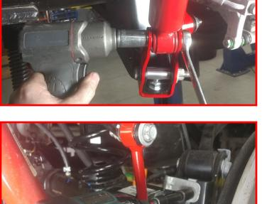
Install the ReadyLIFT brake line bracket to its corresponding side using the provided 1/4" x .75" bolt, washers and nut. Gently rotate/bend the metal brake line until you can line up the locking tab and bolt hole. Install using the factory hardware. Torque all to 5 ft-lbs.
