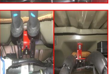
Install the wheels and lower the vehicle to the ground. Torque the lug nuts to the wheel manufacturer specs. Jounce the vehicle a few times to settle the suspension to the new ride height. Torque the upper control arms to 110 ft-lbs, lower control arms and track bar hardware to 135 ft-lbs, and shock and sway bar end link hardware to 50 ft-lbs.
