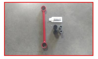
Install the urethane bushings and sleeves into the end links using the supplied grease pack. Use a light amount of grease on the bushing and press into the end link. Use a fair amount of grease on the inside of the bushing and press the sleeve into the bushing.
