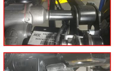
Lower the axle enough to remove the stock spring and rubber isolator. Install the ReadyLIFT spring and factory isolator. Raise the axle enough to hold the springs in place.
