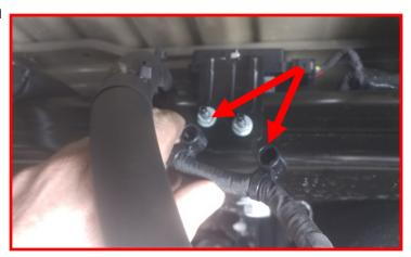
Remove the e-brake cable clamp from the body. Let cables hang. Make sure they are not resting on the locker harness that lays across the frame cross member. When lowering the axle, these cables will become taut and can pinch on the harness.
