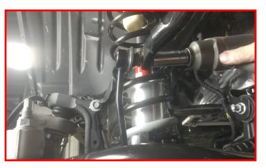
Install the electrical connector that was previously cut to the lower hole in the frame rail. The rest of the harness will hang.
