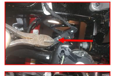
Remove the front sway bar end link from the sway bar. Discard as it will not be reused.
