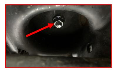
Using the manufactures suggested install instructions, Install replacement performance shocks using factory hardware on top frame mount and provided M12 bolts, washers and nuts.
