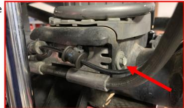
Install the provided 3/8" serrated flange nut to the 3/8" Allen bolt from the under side of the spring perch. Torque to 35 ft-lbs.
