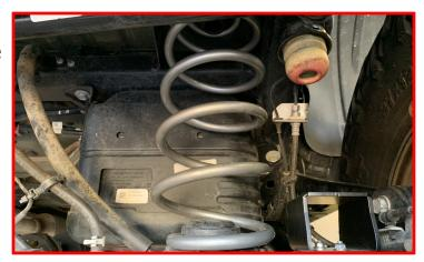
Install the 11" replacement sway bar end link to the axle using the provided 1/2" bolt, fender washer, flat washer and nut.
