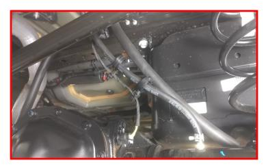
Install the wheels and lower the vehicle to the ground. Torque the lug nuts to the wheel manufacturer specs. Jounce the vehicle a few times to settle the suspension to the new ride height. Torque the upper control arms to 110 ft-lbs, lower control arms and track bar hardware to 135 ft-lbs, and shock and sway bar end link hardware to 50 ft-lbs.
