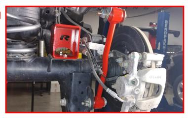
Make sure to have the fender washer to the outside of the end link. Do not tighten at this time.
