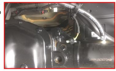
ELECTRIC LOCKER EQUIPPED MODELS ONLY: Clip all remaining clips to the diff vent tube.
