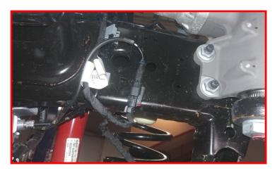
Install the front drive shaft making sure to line up the previous mark using a drop of thread locker and factory hardware. Torque to 40 ft-lbs.
