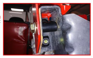
Install track bar into replacement track bar bracket using factory hardware. Do not tighten at this time.
