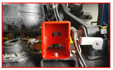
Locate replacement rear track bar bracket and slide over factory axle bracket. Mark center for two 1/2" holes on the outboard side of bracket. Using the appropriate tools drill 1/2" holes through the factory bracket.
