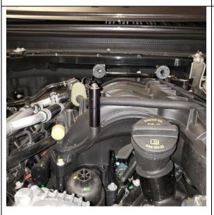
4. Install UPR Catch Can Mounting Bracket on the empty hole on manifold behind oil cap.
