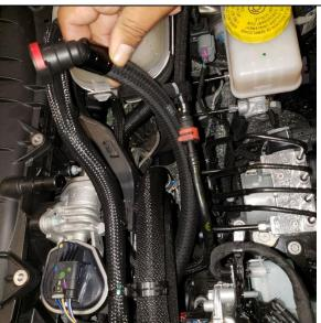
6. Run the Clean Line from the right side of the catch can to the manifold behind the throttle body. You will run the Under your throttle body and coolant overflow line, rotate fittings for best fit. (45° UPR plug n play fitting to the back of cylinder head and 45° fitting to the Catch Can)
