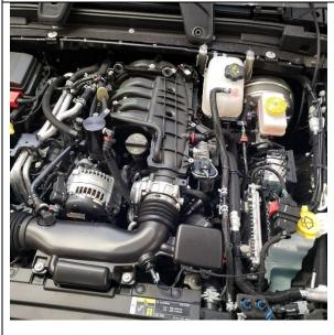
7. Run the Dirty Line from left side of the UPR Catch Can to rear of the passenger cylinder head. (Straight UPR plug n play fitting to the back of cylinder head and 90° fitting to the catch can)
