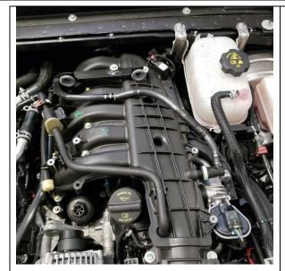
3. Remove PCV line from driver side of engine behind TB (Push Button on fitting to release)
