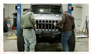
With the help from a second pair of hands, lift the bumper up to the frame of the Jeep and insert the bumper studs into the frame. Using one (1) M10 nut, lock washer, and flat washer per stud, secure the bumper to the Jeep.
