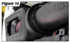
NOTE: Take care not to pinch or trap the pcv line under the tube. Line up the arrows on the filter and tube before tightening all 3 hose clamps.
